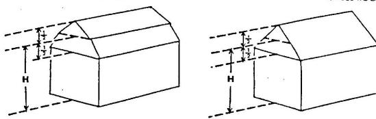
AN ACCESSORY BUILDING OR AN ACCESSORY DWELLING UNIT HEIGHT NOT TO EXCEED TWENTY-FIVE (25) FEET AS MEASURED FROM THE FOUNDATION FLOOR LEVEL TO THE HIGHEST POINT OF THE ROOF SURFACE.
