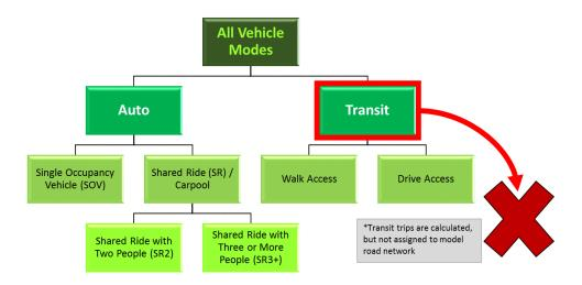
The above chart represents a "Nested Logit Structure," which is a common method in TDFM applications for combining trip results into various vehicular modes. Selecting the appropriate vehicle mode relies on two key factors:
