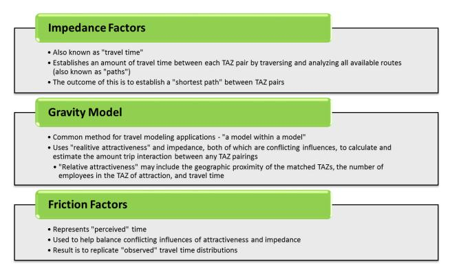
The gravity model is calibrated using successive friction factor adjustments to produce model travel time trip lengths that are consistent with "observed" travel time. Each trip purpose will have a unique travel time trip length and thus, each trip purpose and trip mode must be manually calibrated to ensure consistency with observed travel time data.
