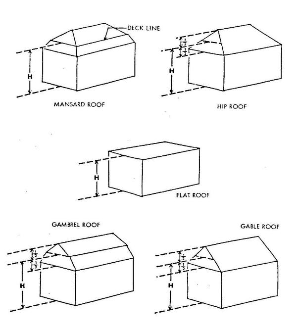
NOTE: GARAGE HEIGHT NOT TO EXCEED 16 FT. AS MEASURED FROM THE FOUNDATION FLOOR LEVEL TO THE HIGHEST POINT OF THE ROOF SURFACE.
